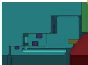
DPE VALVE: Single valve with two seating surfaces, each of which, in the closed position, provides a seal against pressure from a single source.
