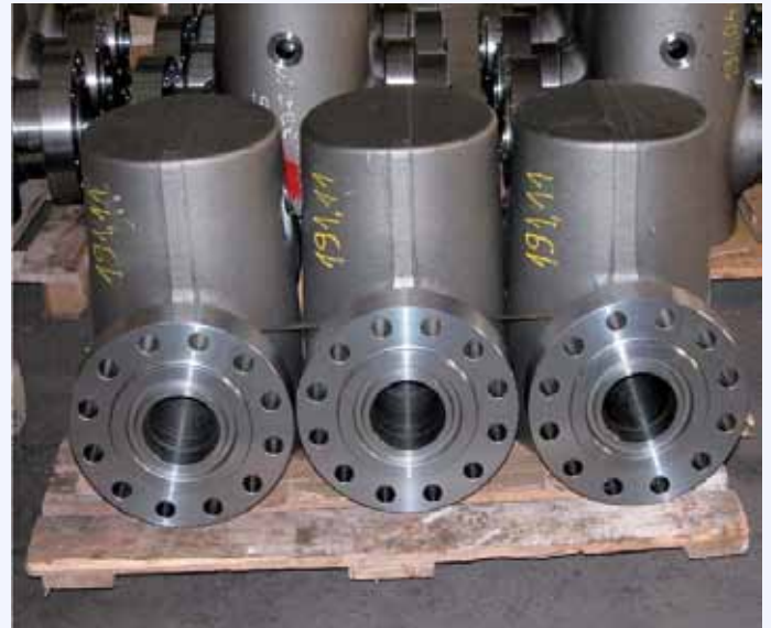
Gate TC Valve Body of 7 1/16" API 10000
