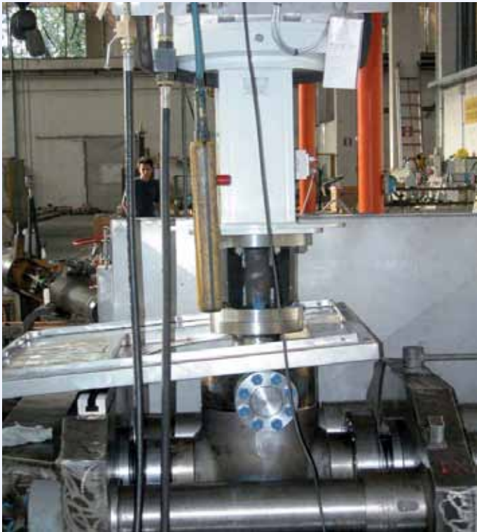
Gate TC 7 1/16" API 10.000 under testing
