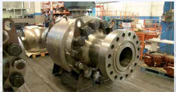
Side Entry Ball Valve 12" API 10000 under assembly
