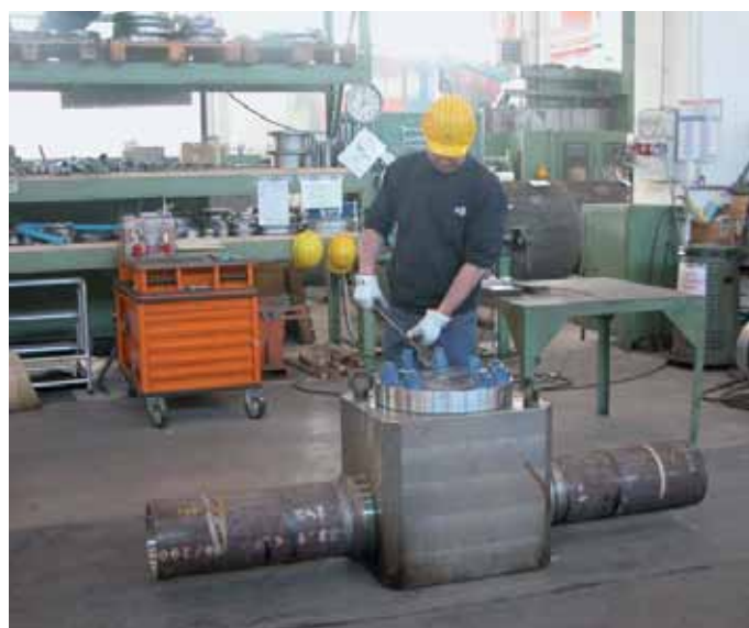
Swing Check API 10000 for Sub Sea application under assembly
