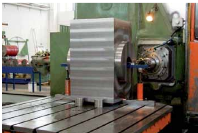
Gate TC Valve Body of 12" API 10000
