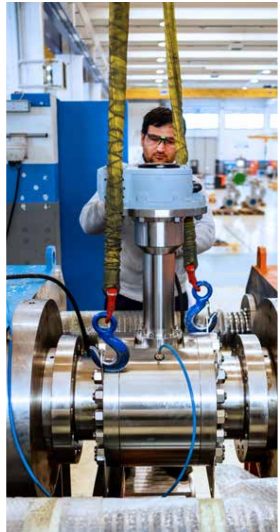
Cryogenic ball valve ready to be pressure tested
